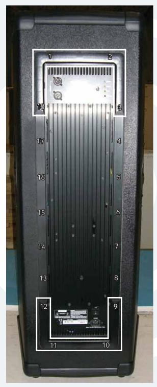
1 Eighteen screws need to be removed from the amplifier assembly using the phillips head screwdriver. The amplifier assembly is capped by two cover plates outlined above.
